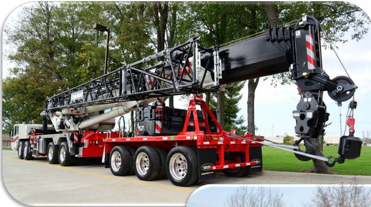
Nelson CBC-30ST shown with a Link-Belt HTC-86110 crane
