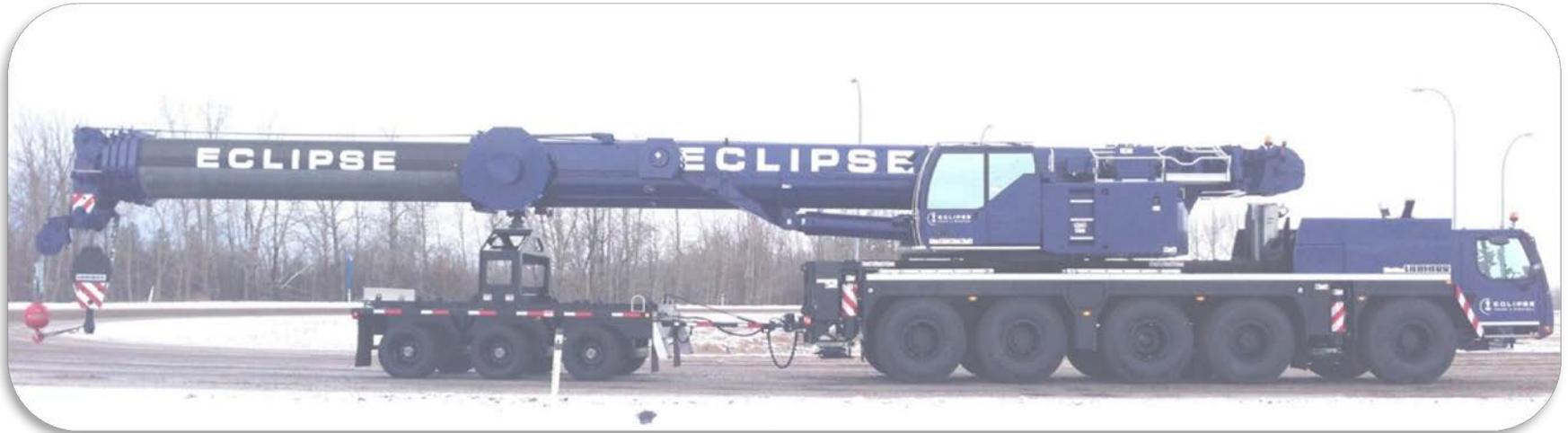
Nelson CBC-30RT shown with a Liebherr LTM-1160-5.1 Crane
