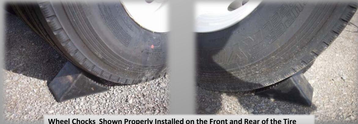
Wheel Chocks Shown Properly Installed on the Front and Rear of the Tire
