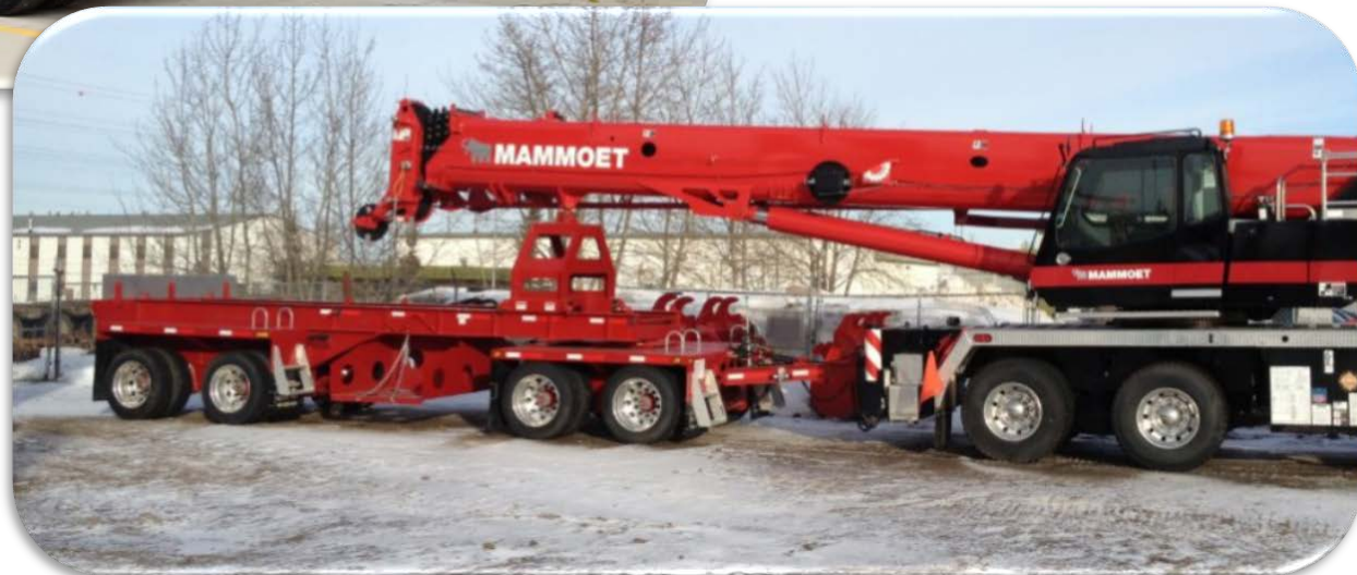
Nelson CBC-40RT shown with a Link-Belt HTC-86100 Crane
