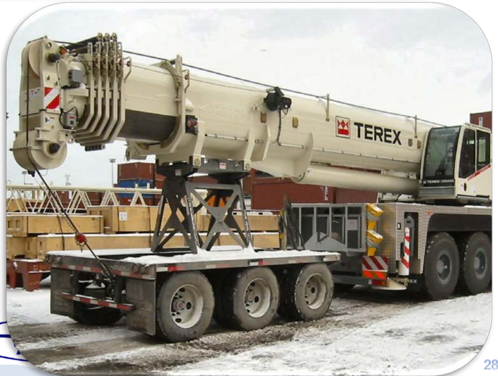
Nelson CBC-30S shown with a Terex AC250 Crane
