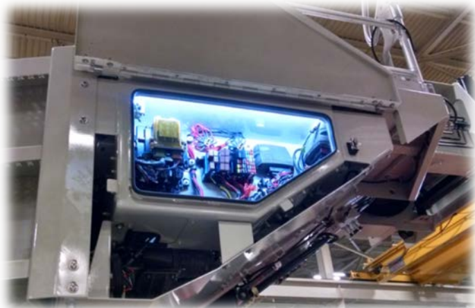
Lights for Electrical Access
