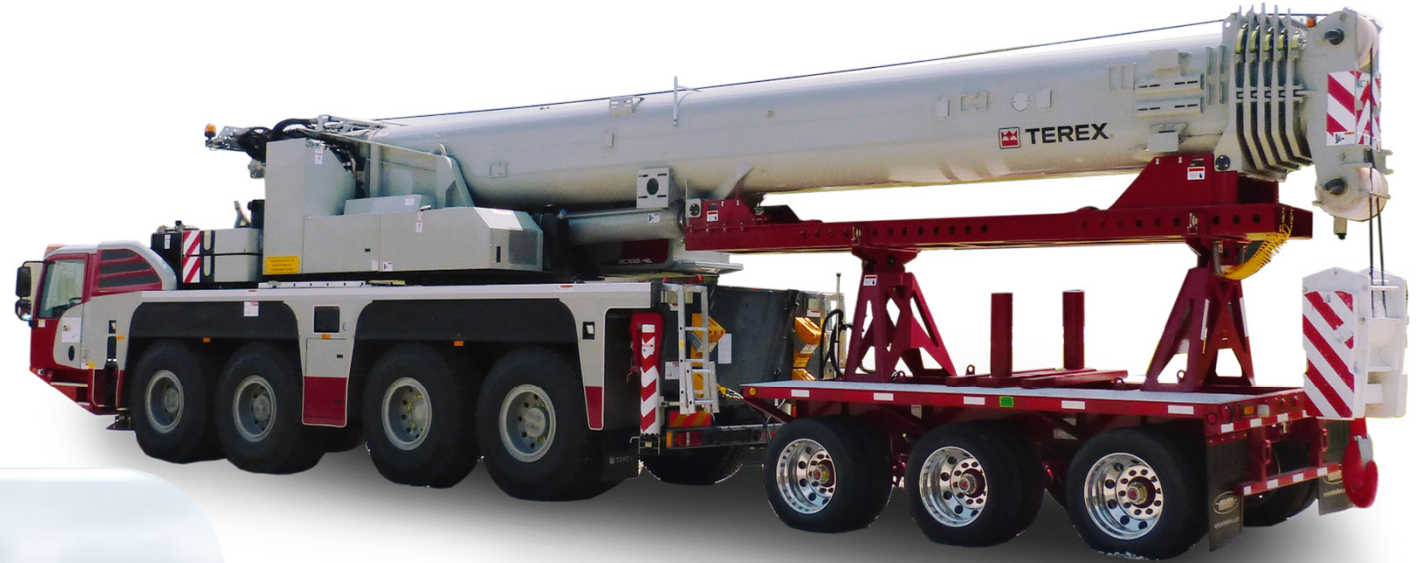
Nelson CBC-30ST shown with a Terex AC100/4L all terrain crane
