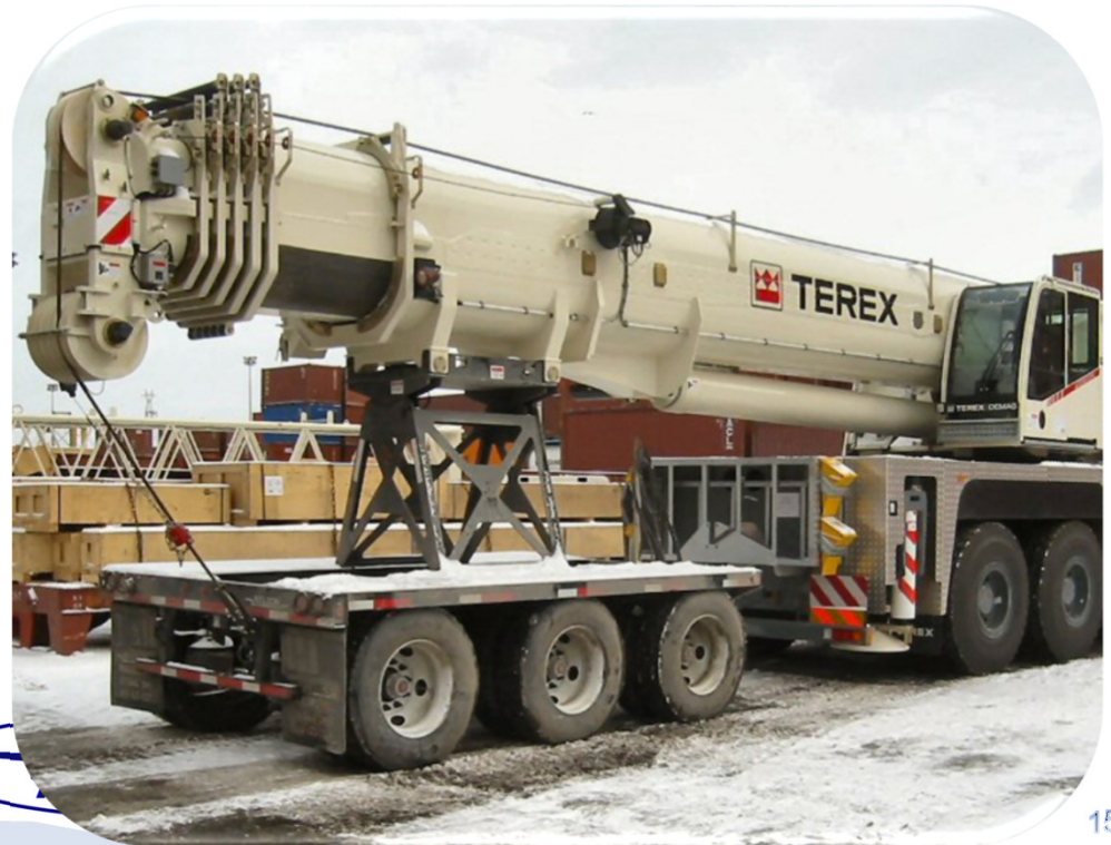
Nelson CBC-30S shown with a Terex AC250 Crane
