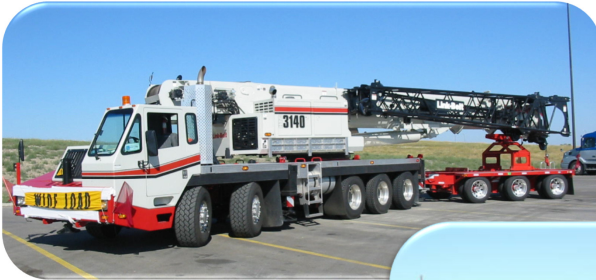
Nelson CBC-30RT on a Link-Belt HTC-3140 Truck Crane
