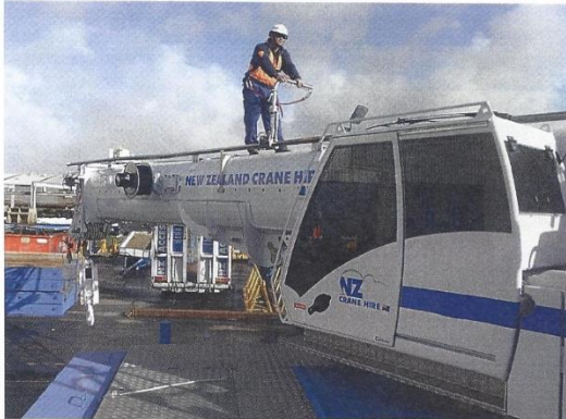
Above: The precise method for fixing the rail to the boom can be different for each crane type, depending on such diverse features as the location of rope retainers and angle of tilt of the cab.
